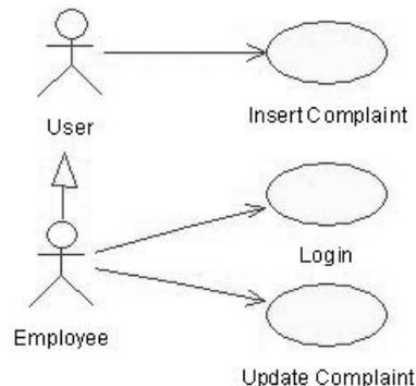
**Figure 5. Use Case Diagram for the Health Watcher System.**
